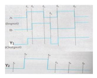
Identify the 'equivalent gate' needed in each case. Show how one can connect an appropriate number of (i) NAND (ii) NOR gates respectively in the two cases to get these 'equivalent gates'.
